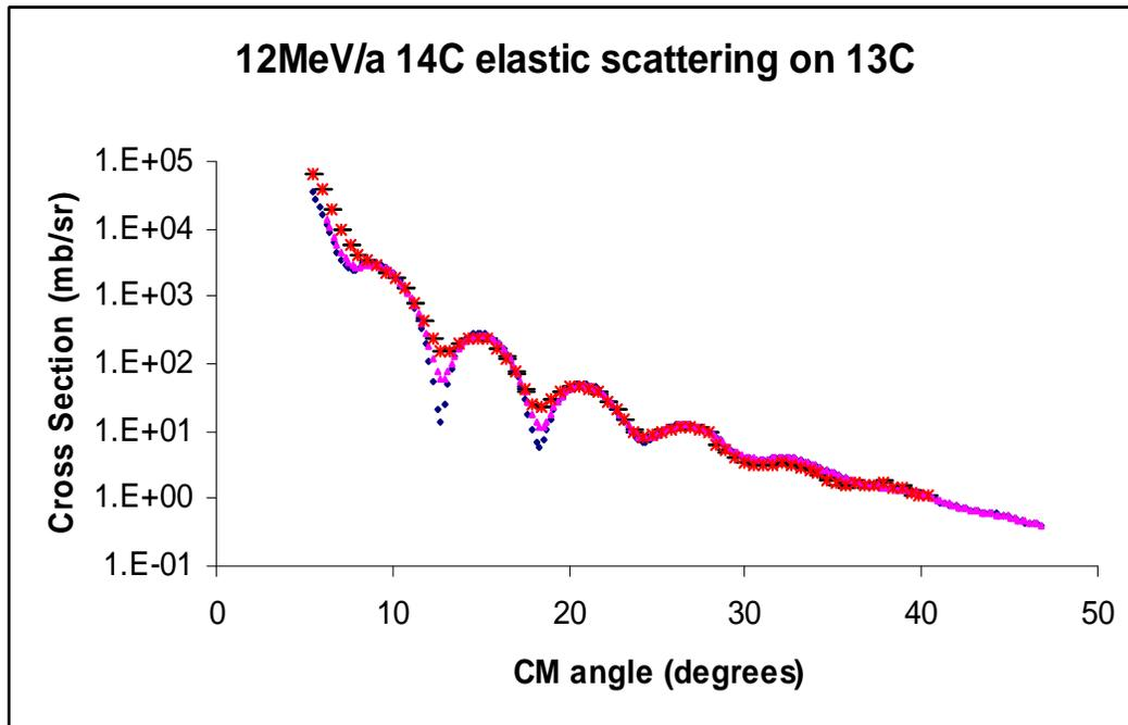
FIG. 1. Elastic scattering of 12MeV/a  $^{14}\text{C}$  on  $^{13}\text{C}$ . The red X's are the measured elastic scattering with statistical error bars shown; the blue squares are the calculation made using an optical model potential and a double folding procedure; the magenta triangles are the same calculation but smoothed using a Gaussian smearing function.
